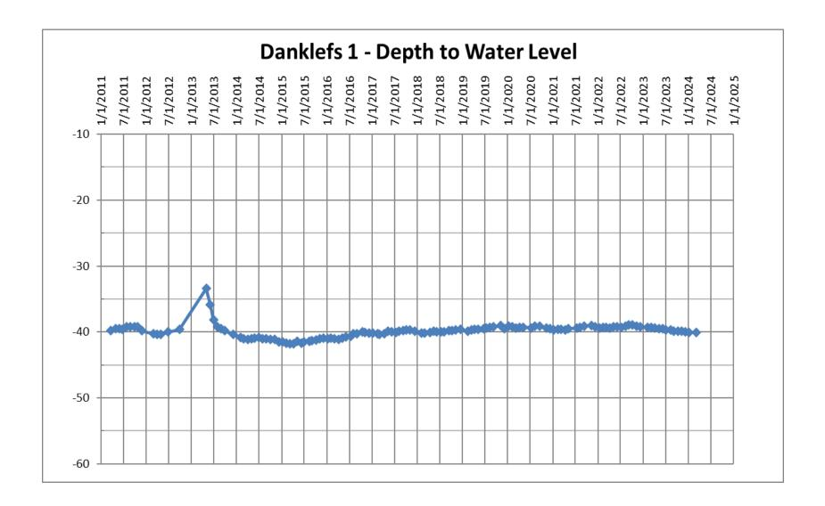
Well Designation: Danklefs 1; State Well #: NA; Well Depth: 46'; Drill Date: unknown; Screen Interval: NA
