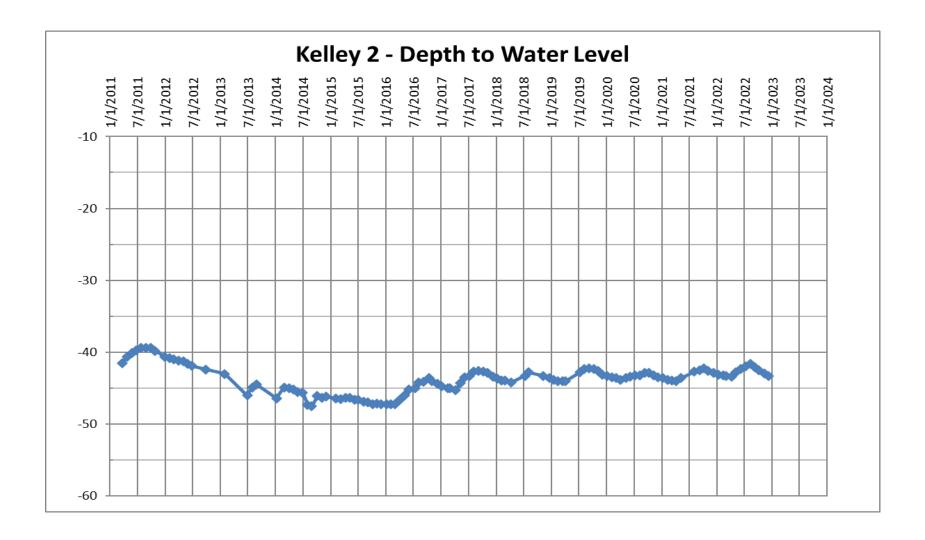
Well Designation: Kelley 2; State Well #: NA; Well Depth: 100'; Drill Date: unknown; Screen Interval: NA
