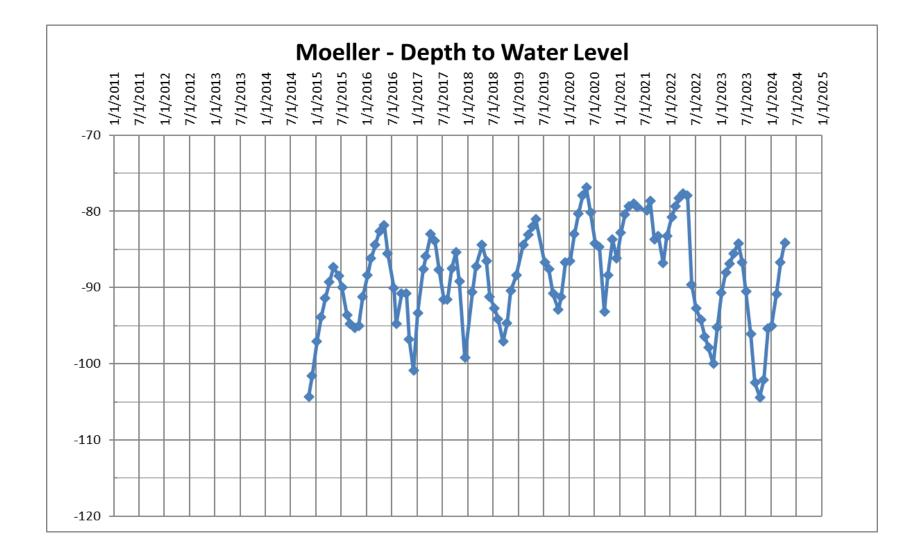
Well Designation: Moeller; State Well #: 6628503; Well Depth: 631'; Drill Date: 11/18/1952; Screen Interval: 240-631'
